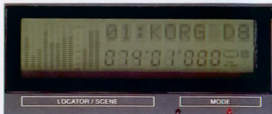
The D8's custom LCD display shows metering (with clip display) as well as song title, location and editing information.
