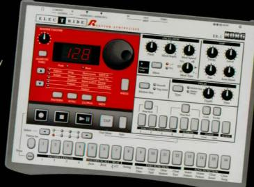
The ELECTRIBE • R can also be controlled from an external sequencer, keyboard, or sampler to function as an analog sound rhythm tone generator, or set up to control or be controlled by other hardware or computerbased sequencers.
