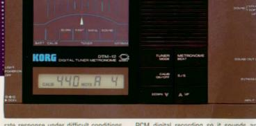
rate response under difficult conditions. Can be used for monophonic instruments and voice training as well as conventional tuning. Produces a tone at the precise pitch of your choice over a four octave range. In the metronome mode you have a choice of 0 to 9 beats to the bar and tempos of from 40 to 208 beats per minute. The metronome sound is a
