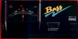
Compact bass tuner with special flat tuning mode allows bass players to easily tune down one half step.
